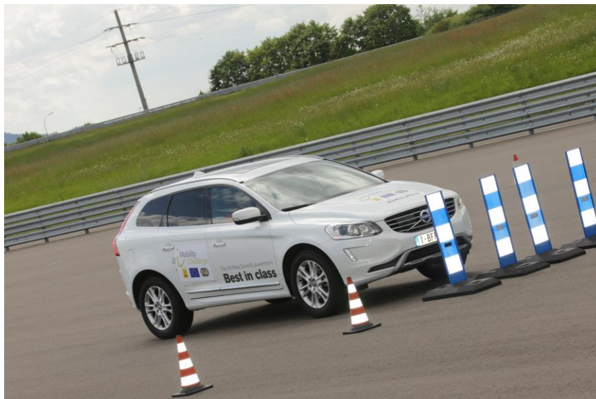
Figure 2. The demonstration of Emergency Braking, the vehicle brakes autonomously in front of an obstacle in case the driver is not reacting on time.
