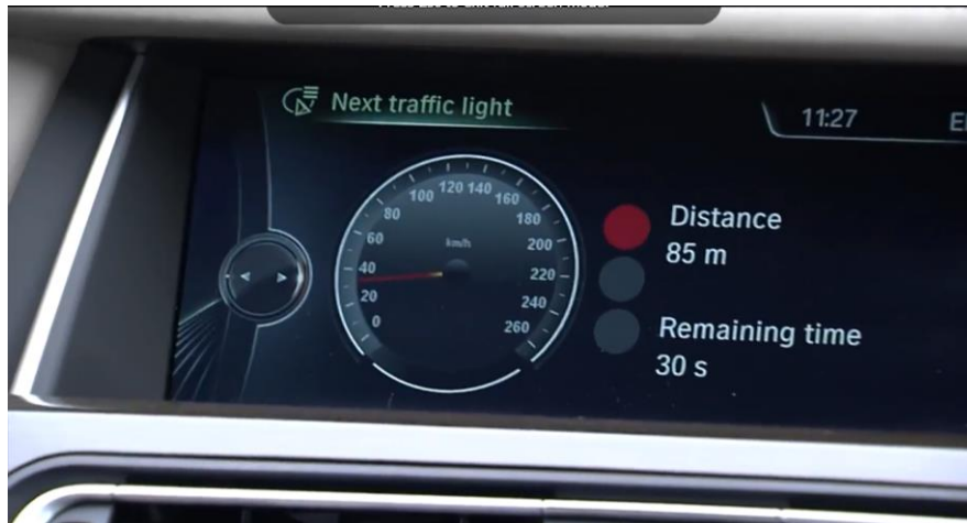
Figure 1. Snapshot of the real time traffic light phasing information provided to the user on his dashboard during the demonstration.
