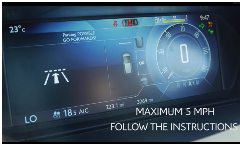
Figure 3. A snapshot of the information provided in the central display screen of the car when using the Park Assist system.
